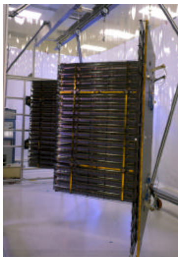
Figure 2: SCARLET Wing in Mid-Deployment
